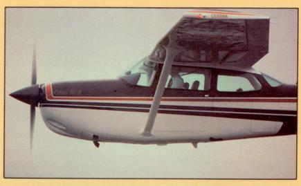
With more power and less drag, the Cutlass can pick up 20 knots over the 172 Skyhawk.
